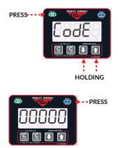
With the gauge off, press and hold both the C LOW and C HIGH buttons, then press the ON/OFF button. Release all three buttons. The gauge will display "CodE".
