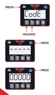
With the gauge off, press and hold both the C LOW and C HIGH buttons, then press the ON/OFF button. Release all three buttons. The gauge will display "CodE".
