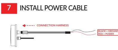
Insert the male connector on the harness onto the female connector on the back of the scale. Make sure to orient the connector properly so that the small cutout on both connectors line up. Once the connector has been pressed in, thread the collar into the scale until it is hand tight.
