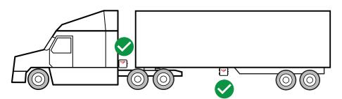
Mount the bracket in the chosen location and install the gauge box to the bracket using supplied hardware.
