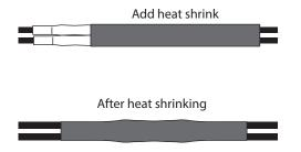
After all connections have been made, heat shrink the entire group of splices so that it seals on the outer jacket of both cables.
