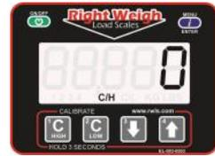
**3:** Use the UP and DOWN arrow buttons to set the desired warning weight. Press and hold the C LOW and C HIGH buttons to save.
