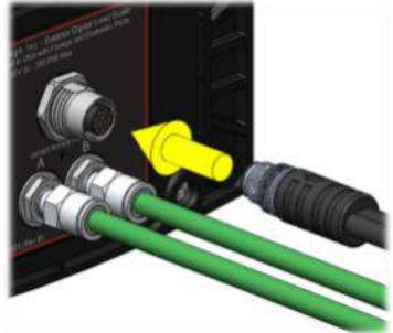
**8:** The additional cable coming out of the 12-pin data connector is used to power the scale and transmit/receive vehicle data. Connect the RED wire to a **SWITCHED** positive (+) power source (**DO NOT connect directly to the battery**) and the BLACK wire to chassis ground (-). The required supply voltage must be between 9 and 32 volts DC.
