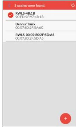
**Step 3:** Select the load scale matching the unique identifier of the scale you wish to sync with. Tap (+)
