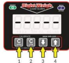
**3:** Press the MENU button, and enter the new 5 digit PIN code using buttons 1, 2, 3, and 4. Press the MENU button again to save the new PIN.
