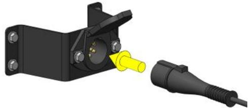
**2:** Connect the other end of the trailer jumper cable to the Right Weigh remote trailer sensor itself.
