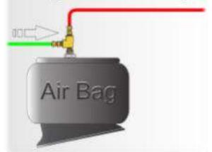
**5:** Insert the new air line into the push-to-connect fitting on the back of the gauge. Repeat steps 2 through 5 for the additional HCV if applicable. Air up the suspension and check connections for leaks.
