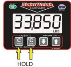
**2:** The display will show the warning value. “0” is the default setting and the display will not flash the weight at any time if it is set to “0”.
