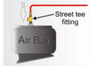
**4:** Install a new 1/4" air line and fitting to be used with the Right Weigh load scale into the street tee. Run the new air line from the street tee fitting to the mounting location of the scale.
