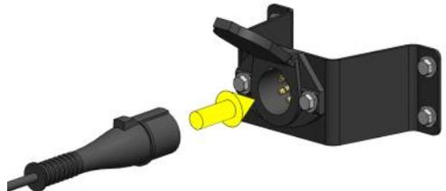
Once connected to a Right Weigh remote trailer sensor, the 201-RTS series load scale will display the weight of the trailer axle group. When disconnected from any remote trailer sensor, the display will read “0” for the trailer axle group.
