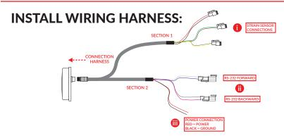
Insert the threaded male connector on the connection harness onto the female connector on the back of the scale. Make sure to orient the connector properly so that the small cutout on both connectors line up. Once the connector has been pressed in, thread the collar into the scale until it is hand tight.
