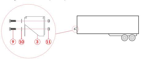
Once the mounting bracket is secure on the trailer, mount the data communication socket to the bracket using the supplied hardware.
